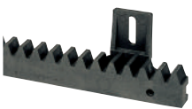
400CN Steel core, fibreglass reinforced, 22x22 nylon rack (Module 4, max 800 kg). Pcs / Pack 10 m
