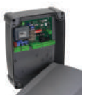
750D770M Electronic control unit for one or two 230 V gate operators with soft-stop and built-in 433,92 MHz rolling code radio receiver, complete with enclosure
