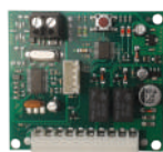
250RXSM2 Self-learning, two-channel, 433,92 MHz plug-in radio receiver. Accepts up to 14 rolling code transmitters
